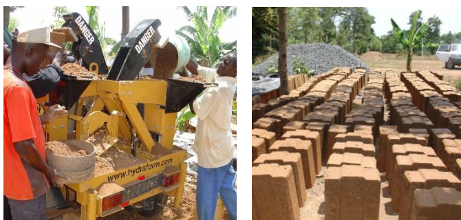
Fig. 12: Production of hydra -form blocks (left side), ready-made hydra-form blocks (right side)
